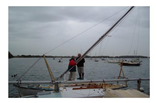
Once the weight of the mast is supported by the stern of the boat, the A frame can be disconnected. The second bolt holding the mast to the tabernacle can be removed and the mast lifted forward to be supported on the pull-pit. This is the only time when a second person is essential. The mast on a Hurley 22 weighs about 100 lbs.
