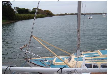
It is handy to have a helper who will look after any tangles with ropes or rigging as the mast is lowered, but all the weight of the mast is supported by the main-sheet. This can be cleated off at any time during the process, so there is no need to rush and the mechanical advantage of using the main-
